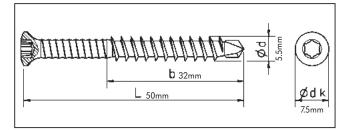
Small countersunk head with under-head pockets.
